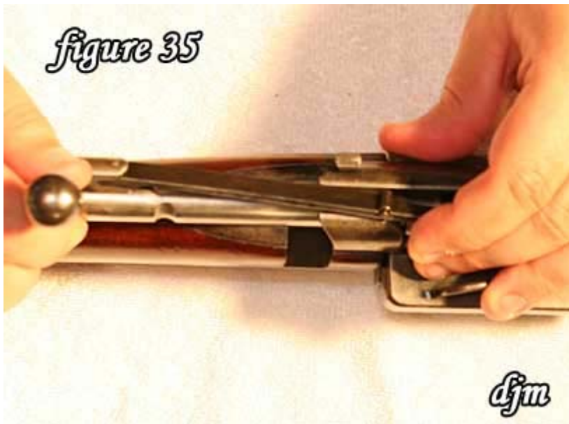
35) Rotate the bolt clockwise while guiding the end of the extractor so it slips into place.
