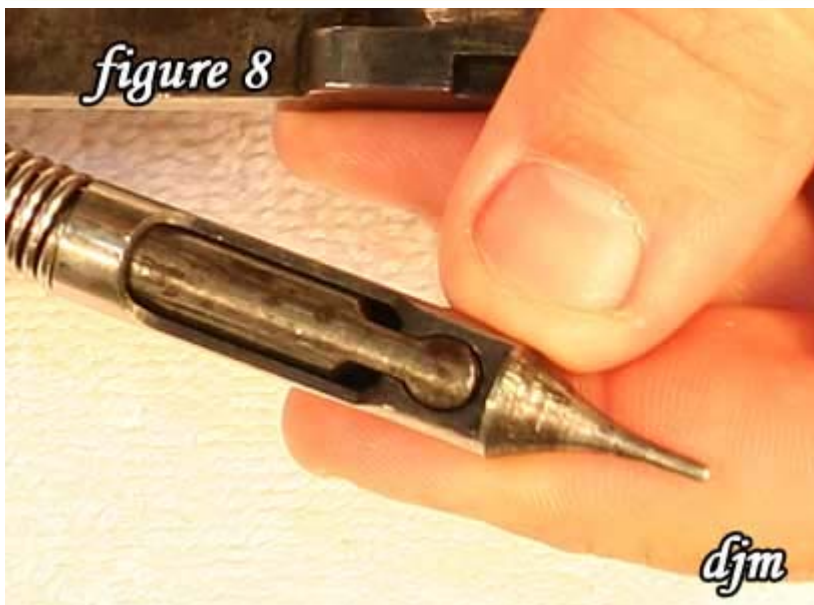
8) Figure 8 shows the striker installed on the end of the firing pin.
