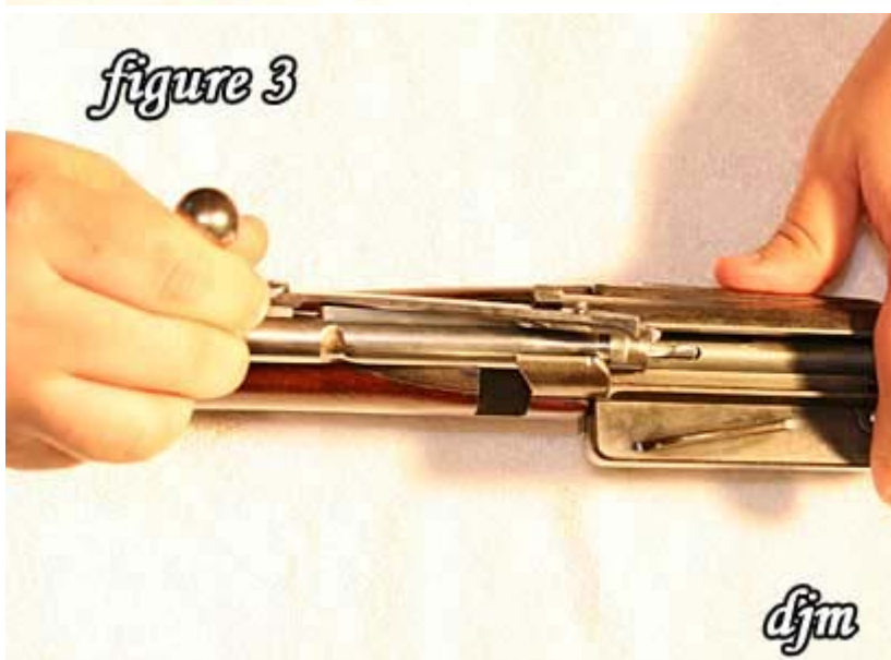
3) With the extractor lifted rotate the bolt to the left. The extractor now clears the receiver.
