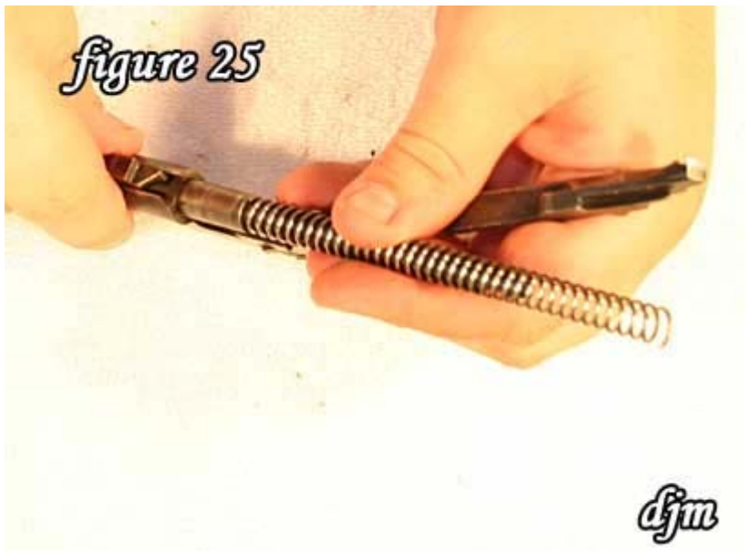
25) Slide main spring over firing pin.
