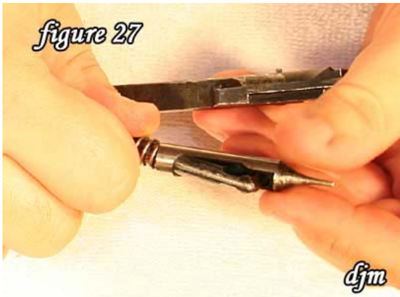
27) With main spring compressed, slide the striker over the firing pin as shown in figure 27.
