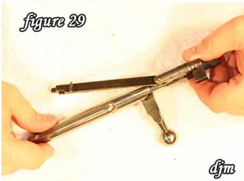
29) Insert the firing pin assembly into the bolt body.
