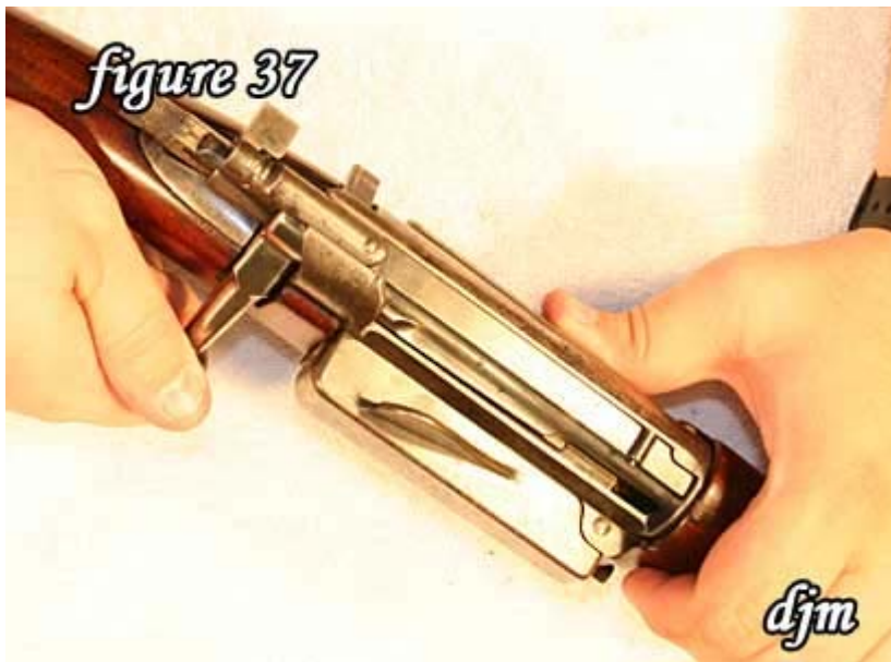
37) Close the bolt and you have completed the disassembly and reassembly of the Krag bolt.
