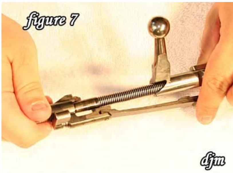
7) Remove the firing pin assembly from the bolt.
