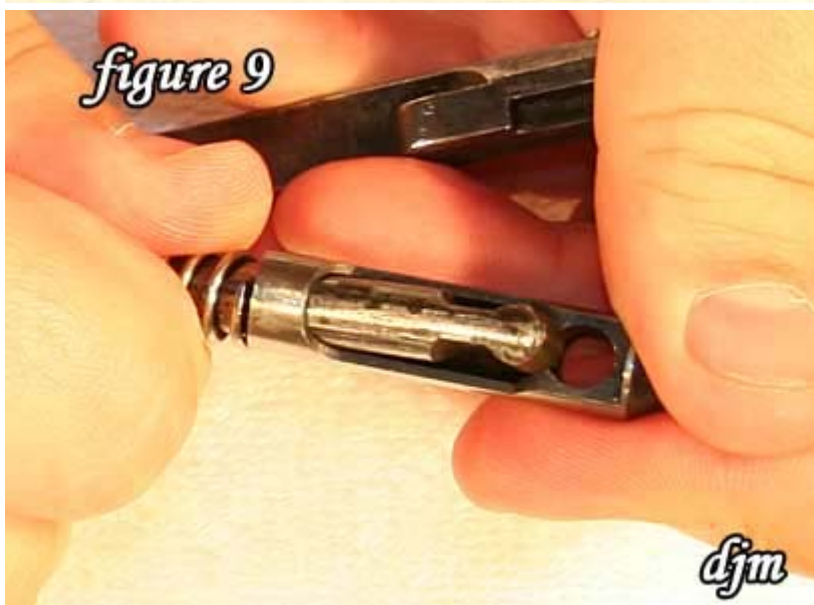
9) Compress the main spring and then pivot back the striker as shown in figure 9.
