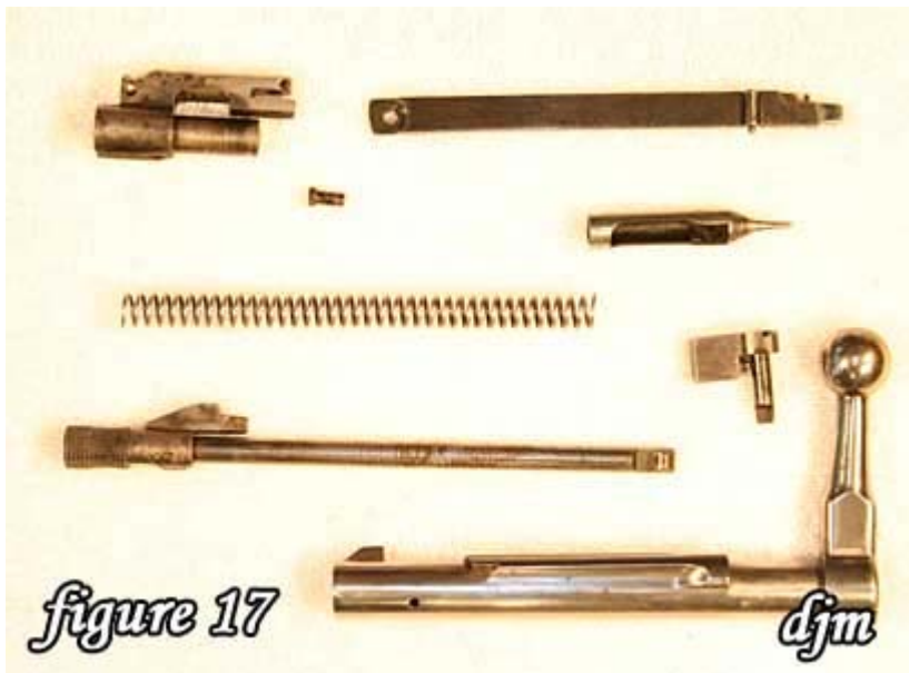
17) Figure 17 shows the disassembled Krag bolt.
